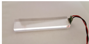
Figure 2: Scintillator tile with SiPM
