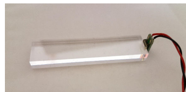
Figure 2: Scintillator tile with SiPM
